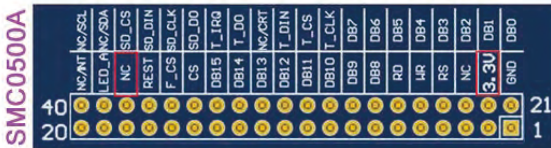
Interface for SMC0500A SSD1963 MCU Parallel TFT LCD Module
